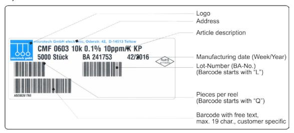
Example for a customer specific label containing barcodes of type Code 128 and Datamatrix:
